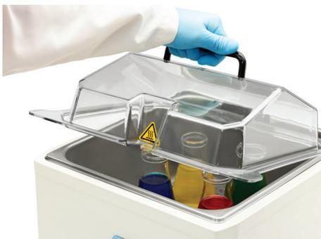
**Enhanced hinge design supports open lid configuration and easy lid removal.**
